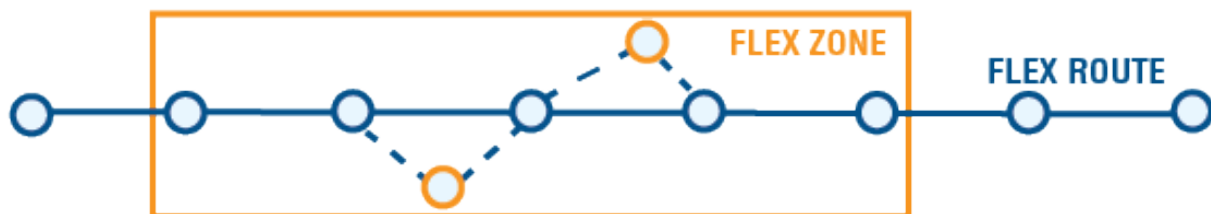
FIGURE 40: FLEX ZONE WITHIN FLEX ROUTE
